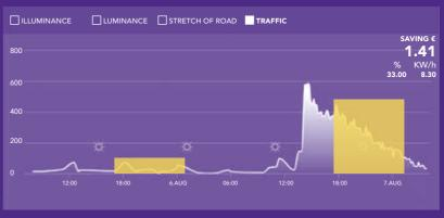
The dashboard shows how the adaptive lighting system adapts to the actual traffic conditions detected on the road. In this case, for example, it can be seen that the adaptive technology operated normally during one night, but adjusted the luminous flux the following night in response to the detection of abnormal night-time traffic (caused by an accident on a neighboring road).
